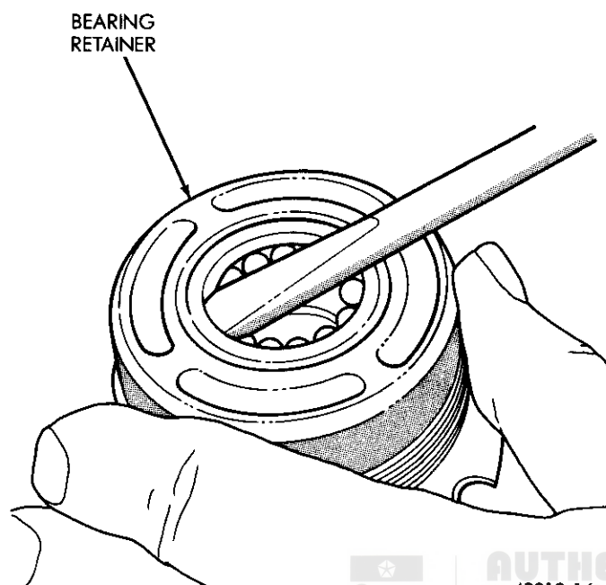
Fig. 7 Wormshaft Lower Bearing Retainer Removal
