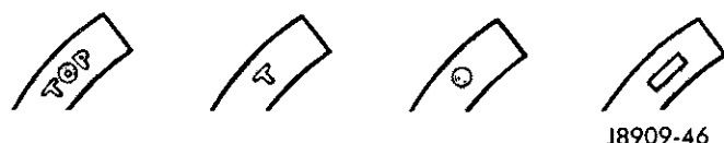
Fig. 68 Top Compression Ring Identification
